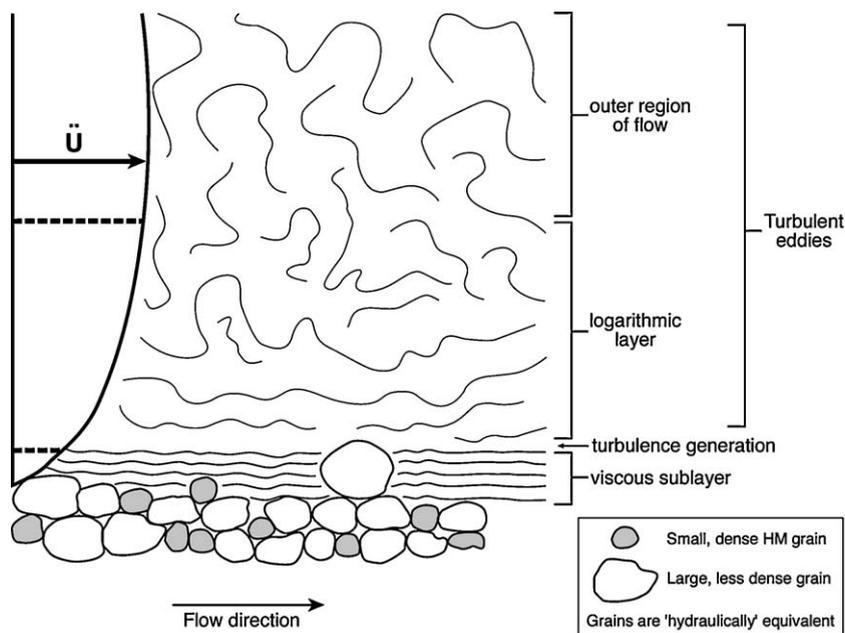
Fig. 1. Definition diagram of turbulent boundary layer.
